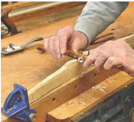
▲ Pic.8 I held the rail between clamp heads, while the 'shave was pulled
